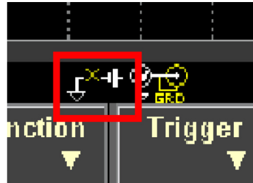
B2985A/87A - voltage source low terminal state
