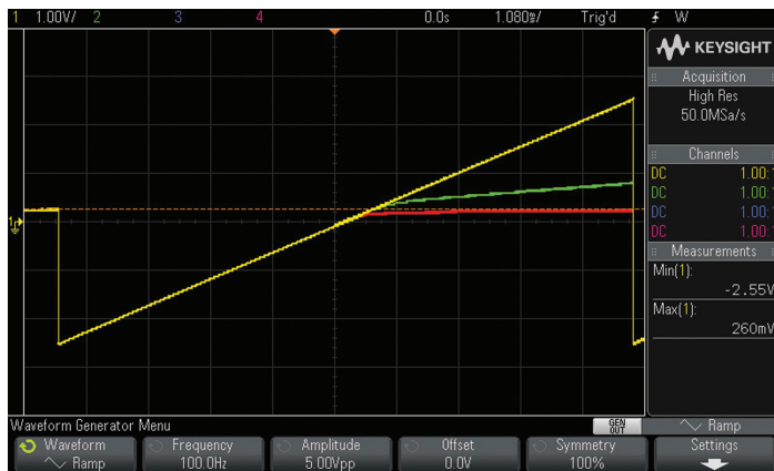
Figure 4. Diode and transistor measurement: without a DUT connected (yellow trace); with a small signal silicon diode as the DUT (green trace); with a power Schottky diode as the DUT (red trace).
