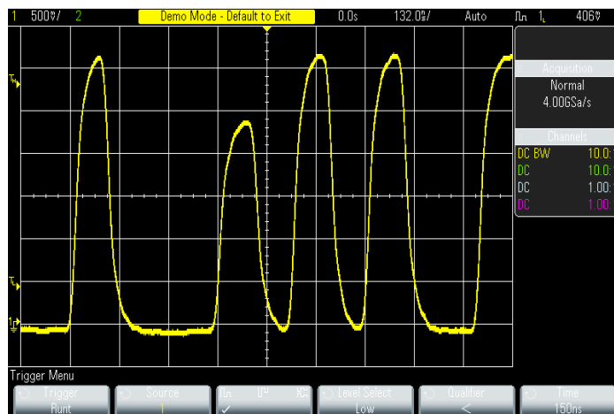
Figure 14. Triggering on a reduced amplitude pulse using Runt triggering.
