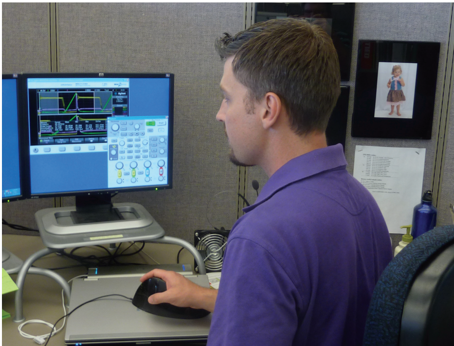
Figure 29. Keysight's InfiniiVision's built-in Web browser with the virtual remote front-panel user interface makes it easy to control and access "live" oscilloscope measurements from anywhere in the world.
