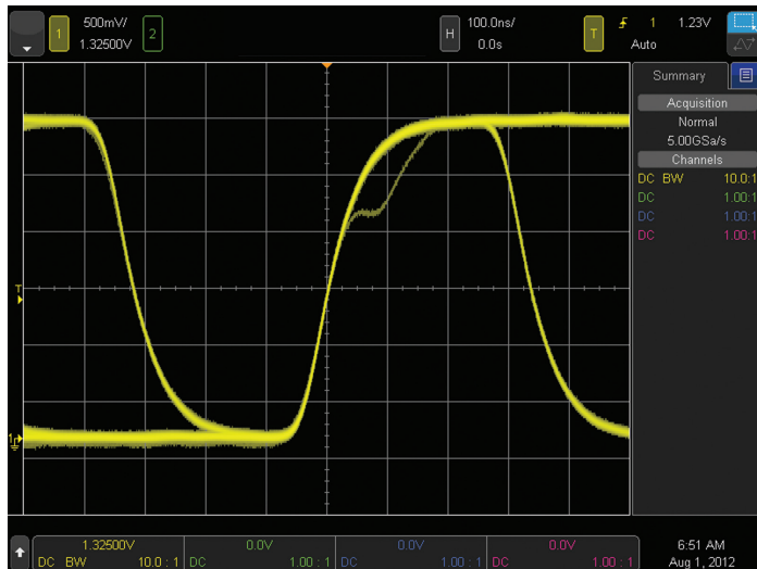
Figure 15. The oscilloscope's fast waveform update rate reveals an infrequent non-monotonic edge.
