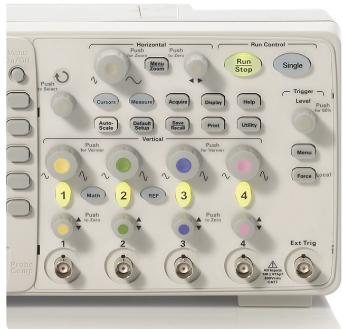
Figure 33. Oscilloscope front panels should include knobs for all key setup variables.
