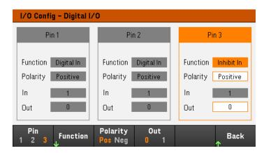
To clear the inhibit protection function, first remove the external inhibit signal. On the front panel select Source Settings > Protection Clear. This will re-enable all dc outputs to their previous states.
