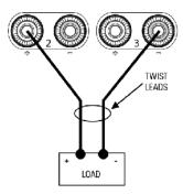
Enable auto-series operation by pressing Output Settings > Operation Mode > Mode Series. The large display indicates a series connection.
