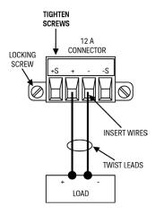
Rear panel (Channel 1 example) 12A max current (accepts wire sizes from 12 to 30 AWG).
