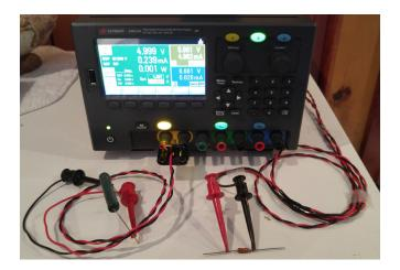
It is good engineering practice to twist your wires to reduce lead inductance and reduce noise pickup. In the test example shown above, Channel 1 is set up for 2-wire operation using a single twisted pair. Channel 2 is set up for 4-wire operation using a twisted pair for the output leads and a separate twisted pair for the remote sense leads.
