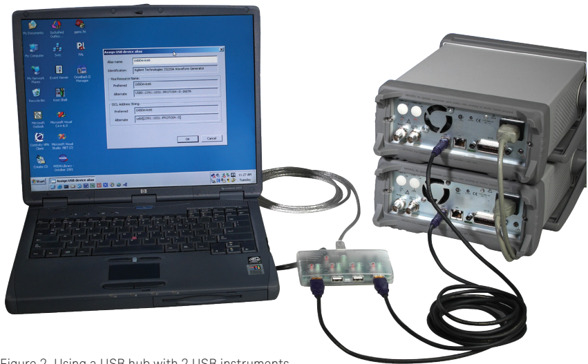
Figure 2. Using a USB hub with 2 USB instruments
