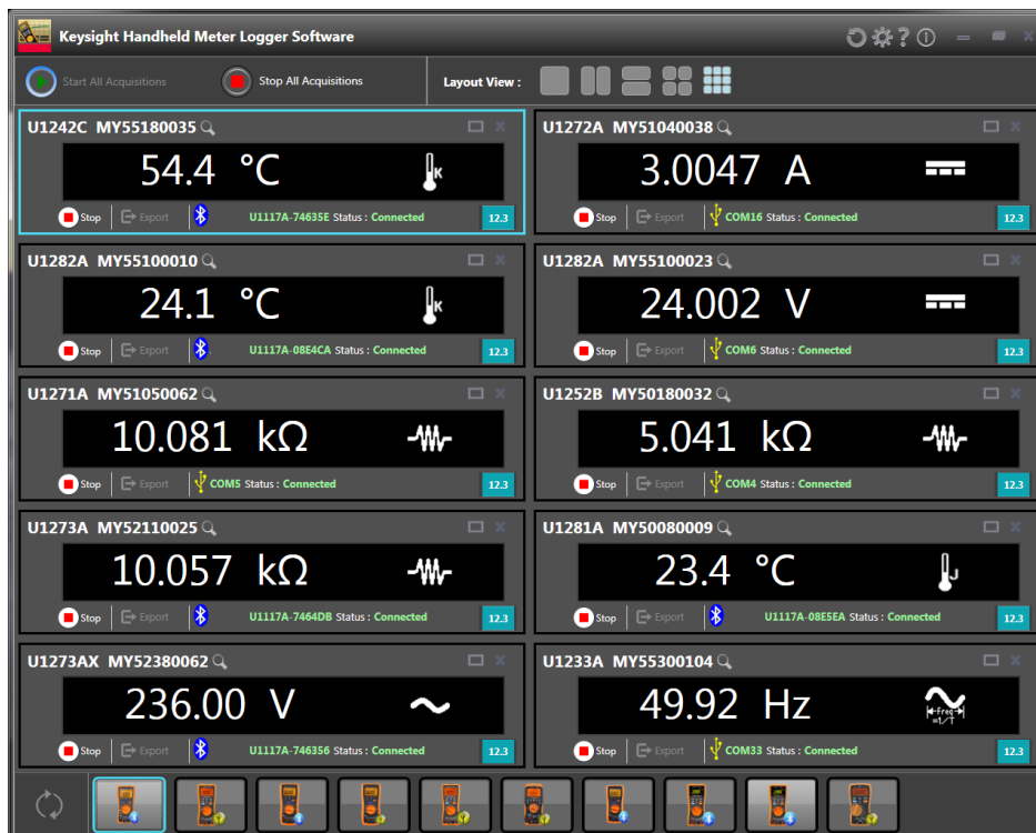
Figure 2. Ten U1200 series handheld multimeters connect to Keysight Handheld Meter Logger Software
