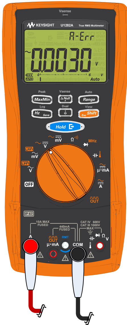
Figure 1-2 Example of A-Err for wrong terminal input
