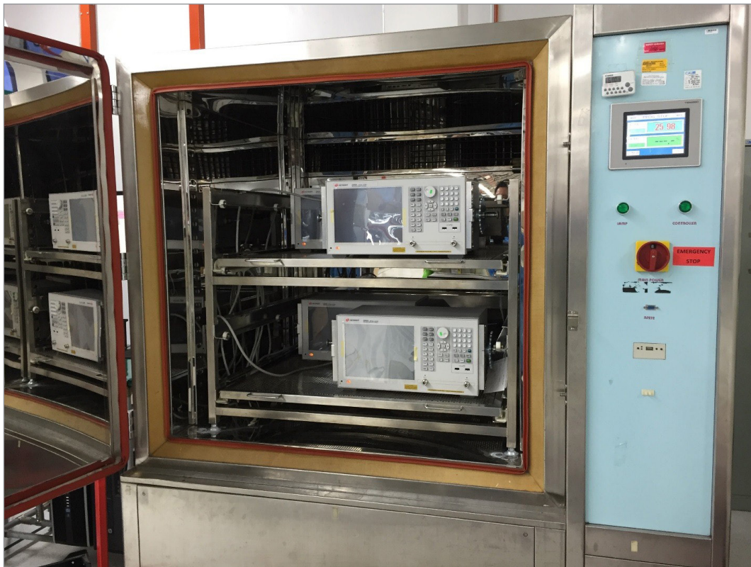
Figure 1. An example of a large oven with multiple products tested simultaneously
