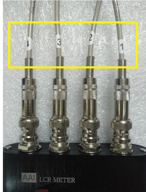
Figure 5-2 Four-wire Kelvin clamp
