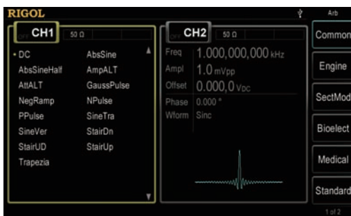
Arbitrary waveform function and built-in 150 waveform
