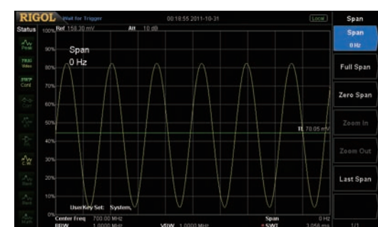
Zero span to demodulate the AM signal
