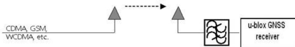
**Figure 22: Measures against in-band jamming**
