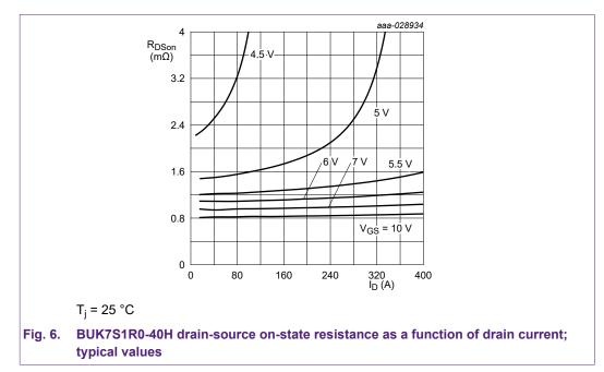
The data provided in Fig. 6 is for 25 °C and is only for  $I_D$  up to 400 A. Therefore, it cannot be used for  $I_{DM}$  estimation. As  $R_{DSon}$  dependence on  $I_D$  is not taken into account, the data on Fig. 5 is an over estimate. Actual measurement of the device capability is a better way to determine with confidence the current handling capability at various time intervals.
