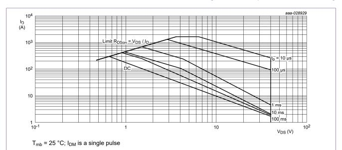
Fig. 11. BUK7S1R0-40H Safe operating area; continuous and peak drain currents as a function of drain-source voltage
