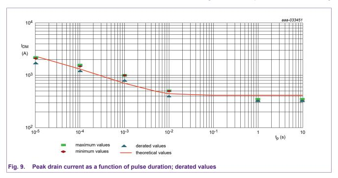
Consequently, the characteristic curve is a theoretical line which is supported by test results. If the derated minimum measured values are above the theoretical line then the theoretical line is the limit, otherwise the derated measurement point will determine the characteristic; see Fig. 10
