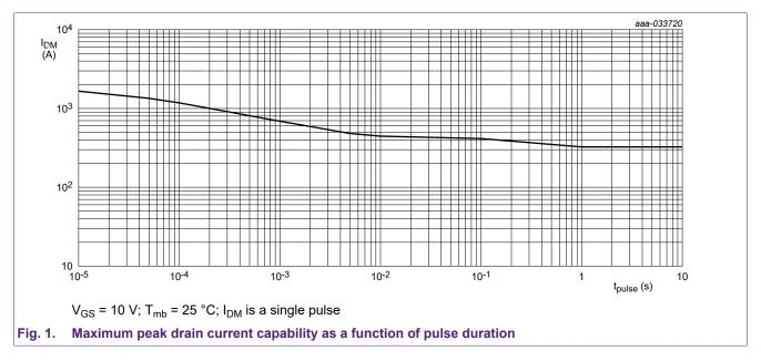
In Fig. 1 time is shown logarithmically from 10  $\mu$ s to 10 s. The maximum allowed peak drain current  $I_{DM}$  is also expressed logarithmically.
