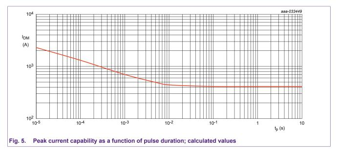
The maximum theoretical device current for a 10  $\mu$ s pulse is 2.3 kA, see <u>Fig. 5</u>. However, the R<sub>DSon</sub> changes with I<sub>D</sub> and this is not taken into account with this approach. R<sub>DSon</sub> value increases with I<sub>D</sub>. See the example graph from BUK7S1R0-40H data sheet in <u>Fig. 6</u> below:
