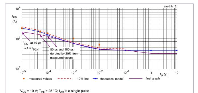
Fig. 12. BUK7S1R0-40H peak drain current capability; measured values, theoretical model, 10% line and final graph
