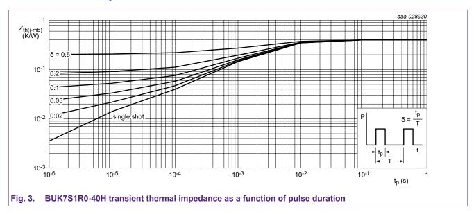
The transient power capability characteristic as a function of time can be determined, assuming that the MOSFET junction temperature would be raised by 150 K, from 25  $^{\circ}$ C to 175  $^{\circ}$ C. See Eq. 1 and Fig. 4.
