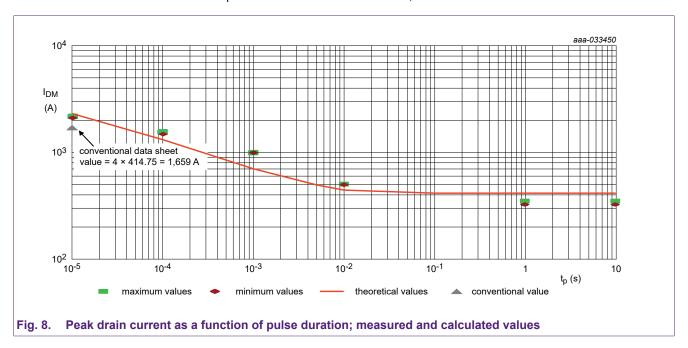
Considering a small sample of measured devices,  $I_{DM}$  at 10  $\mu$ s achieves around 2.1 kA. As previously suggested, this is less than the value derived on Fig. 5 of 2.3 kA. Fig. 8 demonstrates the relationship between the theoretical and measured values for  $I_{DM}$ . The grey triangle denotes the value obtained by convention.
