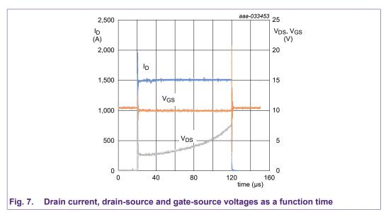
In this example a 1,500 A, 100  $\mu$ s pulse is applied to a device which is already switched on. Initially the voltage drop across the device is around 2.7 V, therefore  $R_{DSon}$  is around 1.8  $m\Omega$
