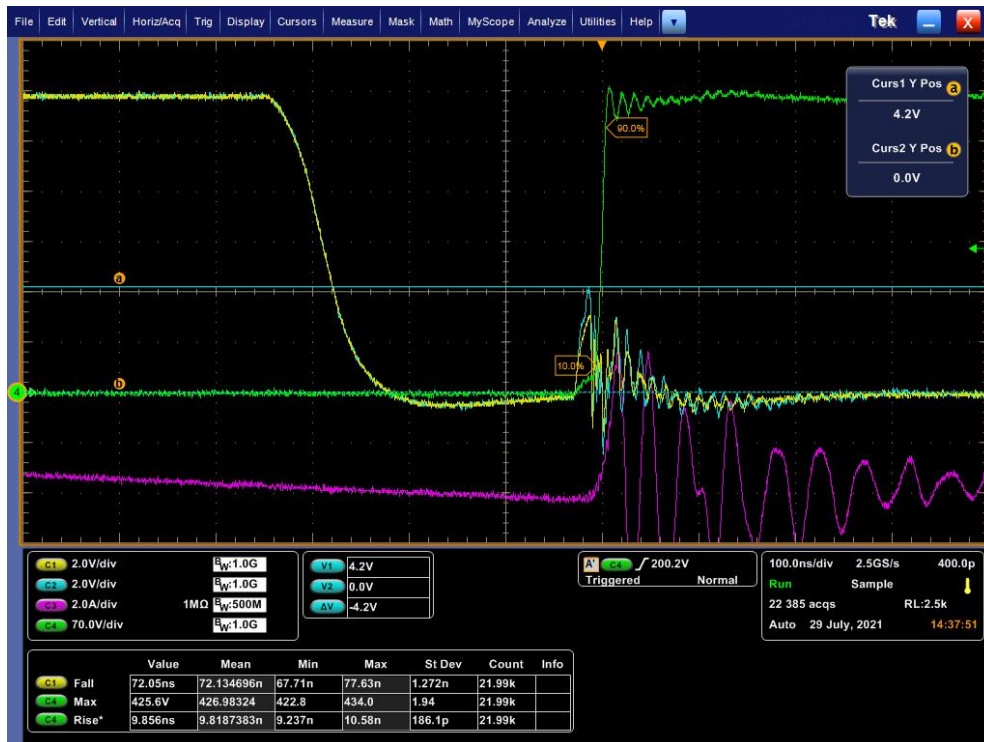
Fig. 10. Zoom of Q2 and Q4 low-side GaN FETs - switch ON
