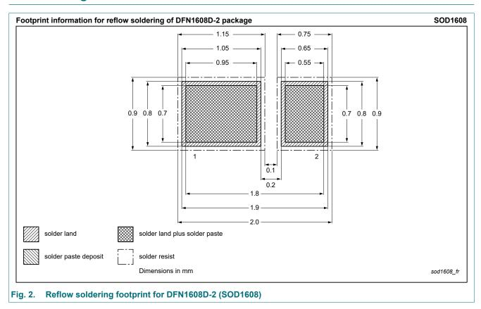
plastic, leadless ultra small plastic package with side-wettable flanks (SWF); 2 terminals; 0.94 mm pitch; 1.6 mm x 0.8 mm x 0.37 mm body
