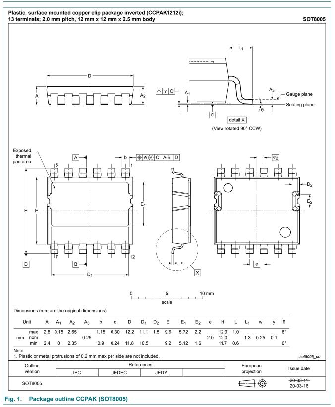
Plastic, surface mounted copper clip package inverted (CCPAK1212i); 13 terminals; 2.0 mm pitch, 12 mm x 12 mm x 2.5 mm body
