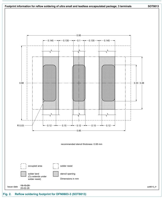
DFN0603-3; plastic, ultra small and leadless full encapsulated package; 3 terminals; 0.225 mm pitch; 0.63 mm x 0.33 mm x 0.25 mm body
