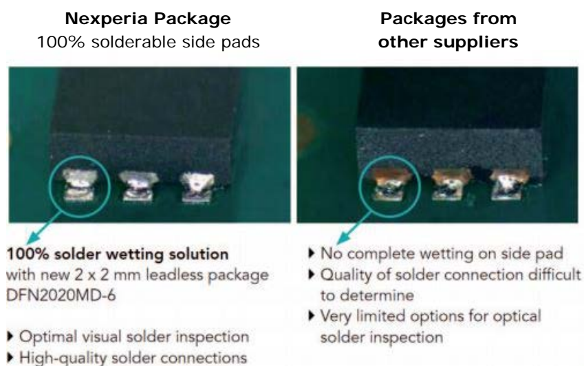
Fig. 1: Comparison of packages with and without tin-plated side pad
