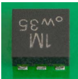
Fig. 26: DFN2020-6 (SOT1118) Component D263 without wettable side pads
