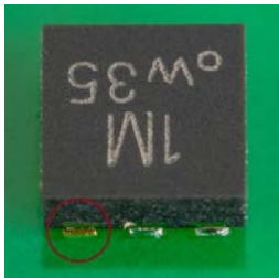
Fig. 18: DFN2020-6 (SOT1118) without wettable side pads (8-D260): Solder paste printing with fails
