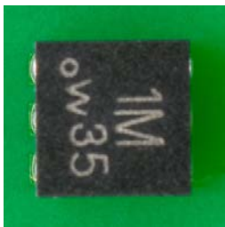
Fig. 13: DFN2020-6 (SOT1118) without wettable side pads (2-D294): Solder paste printing without fails
