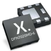
Fig. 5: DFN2020MD-6 (SOT1220) with tin-plated wettable side pads
