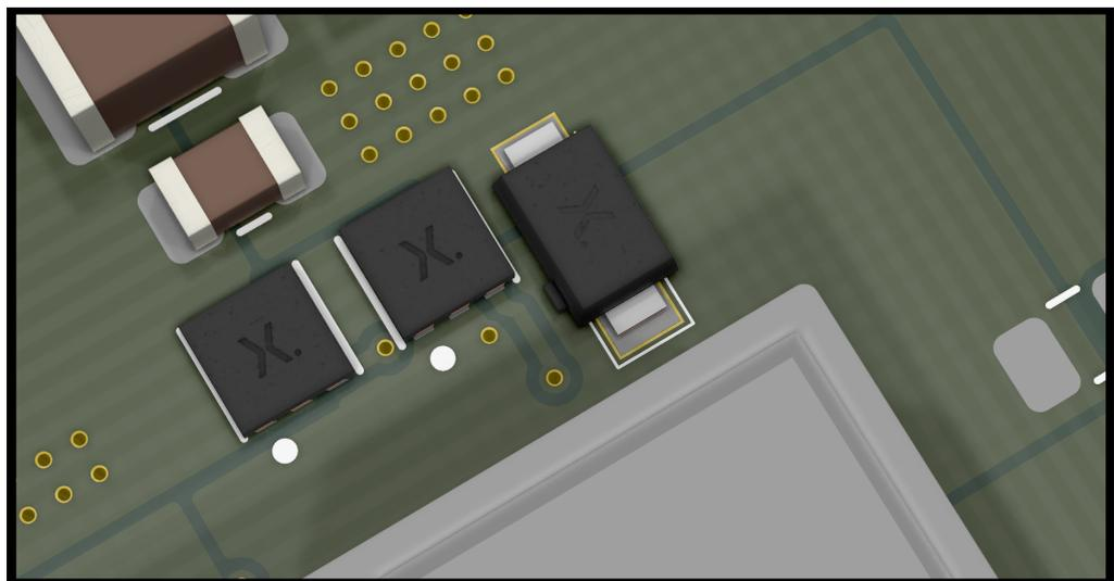
Fig. 10. Buck converter PCB layout: top side detail showing MOSFETs and Schottky diode
