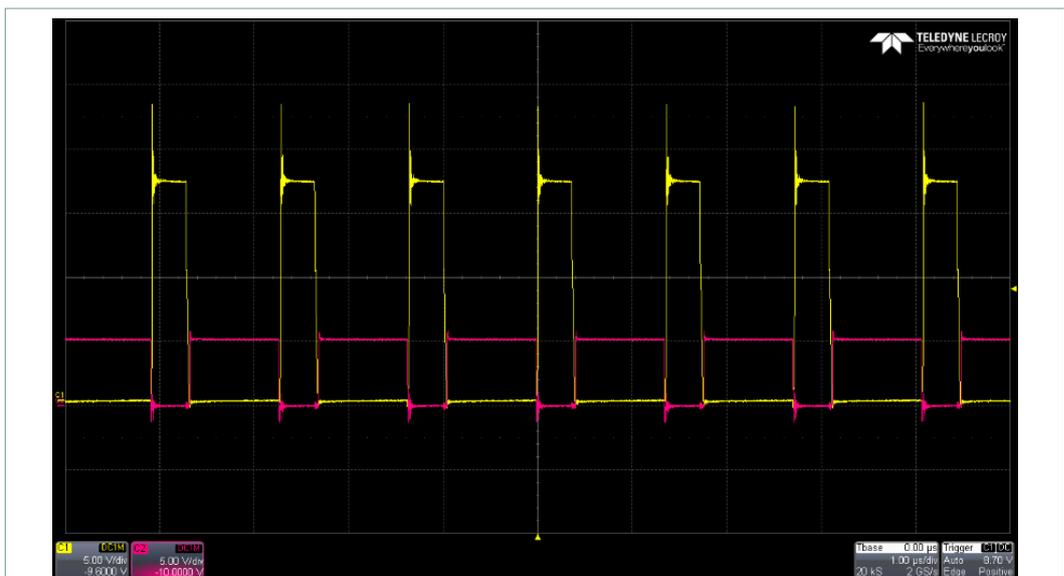
Fig. 13. Continuous mode gate waveforms: high-side (yellow), low-side (pink)
