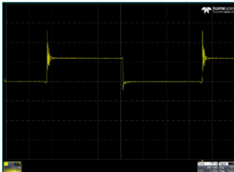
$$I_l = 4 \text{ A}; V_{\text{out}} = 3.3 \text{ V}; f = 750 \text{ kHz}$$
