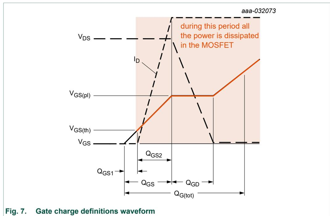
**Fig. 7. Gate charge definitions waveform**
