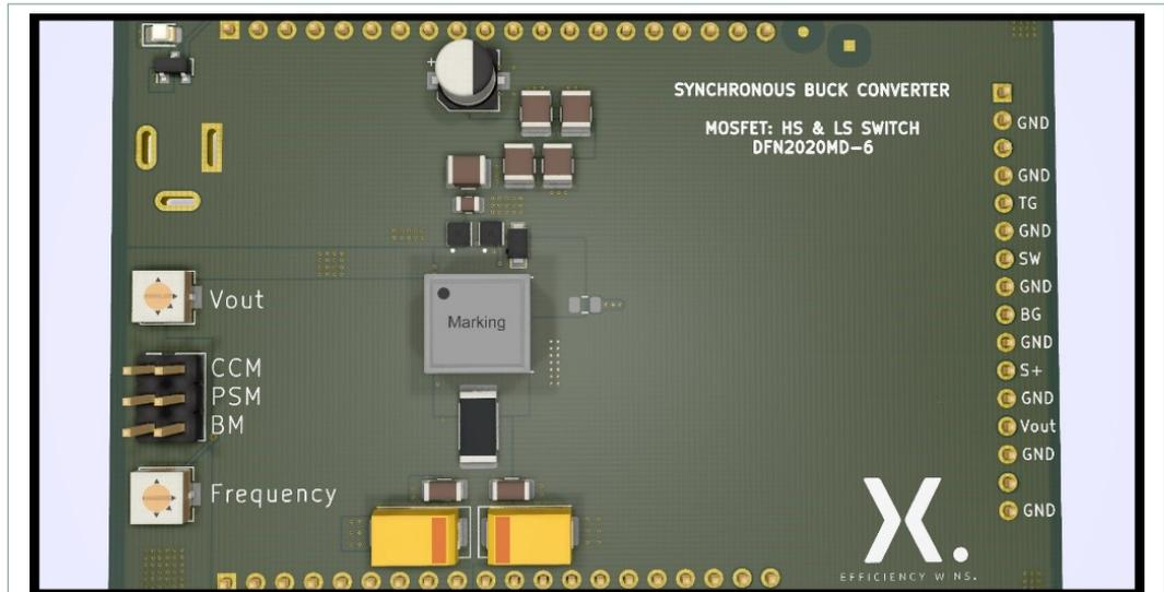
Fig. 9. Buck converter PCB layout: top side
