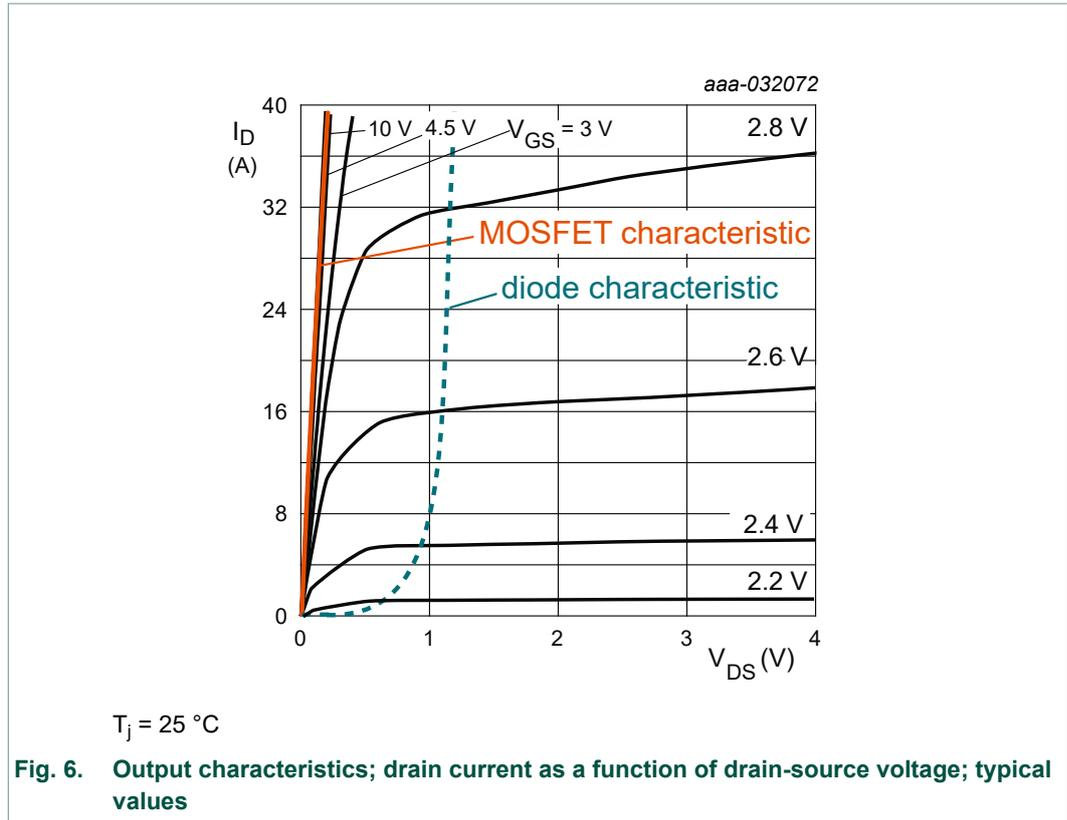
This difference in forward voltage drop means that the conduction losses of a low-side switch would be reduced by a great amount. This is especially important if the application is in the medium to high power segment.
