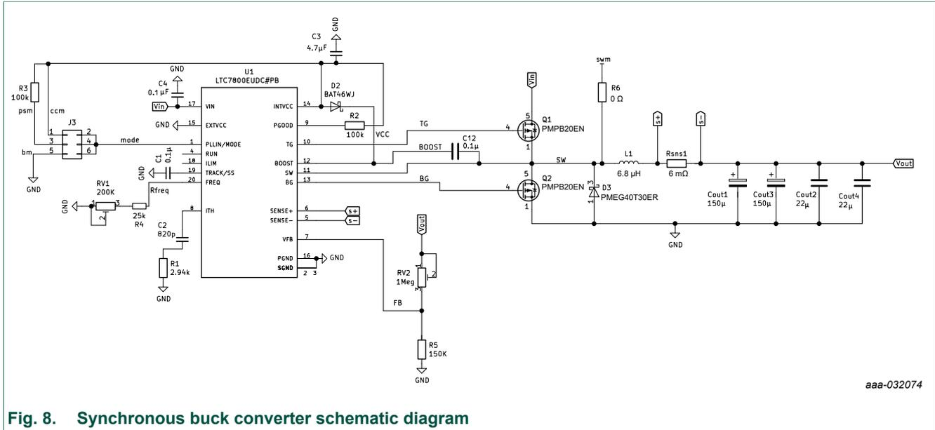
Fig. 8. Synchronous buck converter schematic diagram
