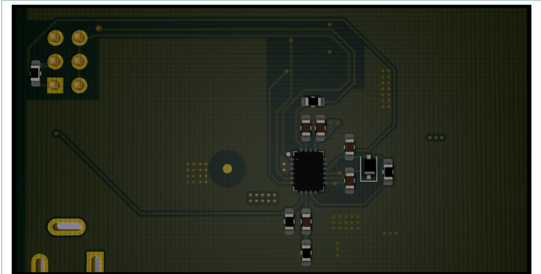
Fig. 12. Buck converter PCB layout: bottom side detail showing controller IC
