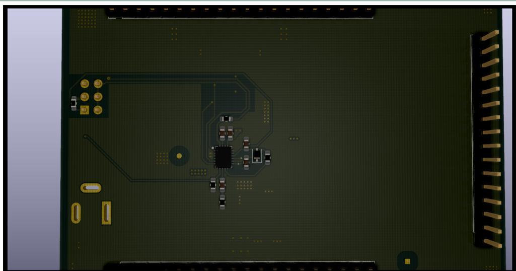
Fig. 11. Buck converter PCB layout: bottom side
