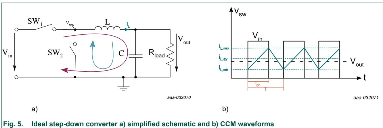
**Fig. 5. Ideal step-down converter a) simplified schematic and b) CCM waveforms**
