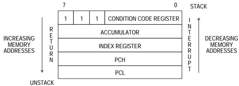
NOTE: Since the stack pointer decrements during pushes, the PCL is stacked first, followed by PCH, etc. Pulling from the stack is in the reverse order.
