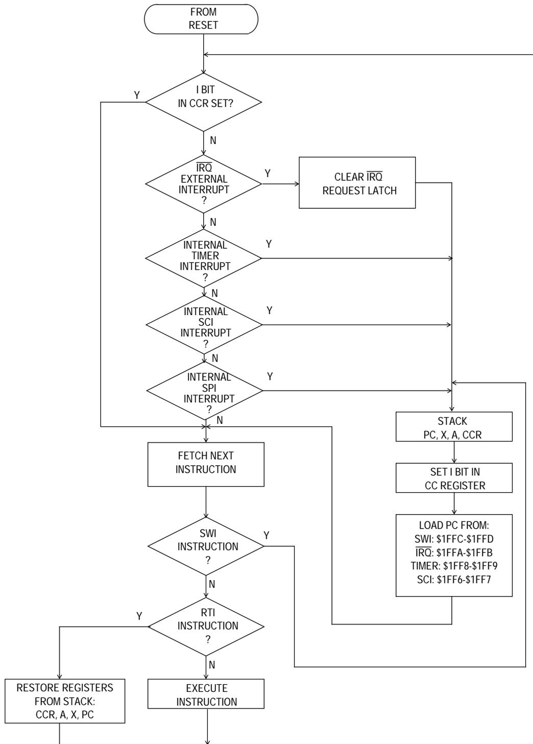
**Figure 4-1. Interrupt Flowchart**
