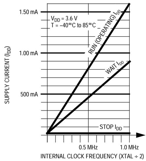
**Figure 13-3. Maximum Supply Current Versus Internal Clock Frequency, V<sub>DD</sub> = 3.6 V**
