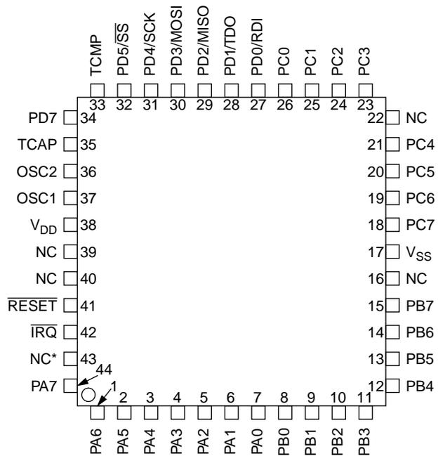
\* If MC68HC705C4A OTPs are to be used in the same application, this pin should be tied to  $V_{DD}$ .
