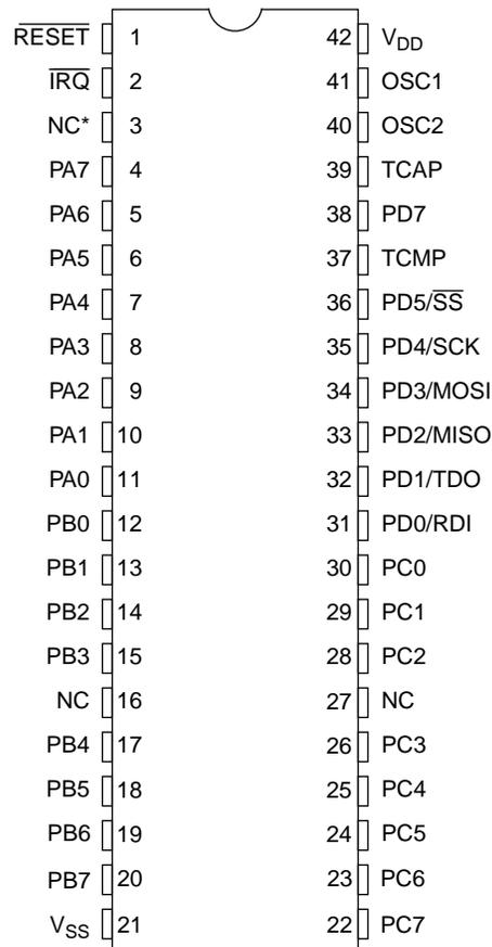
\* If MC68HC705C4A OTPs are to be used in the same application, this pin should be tied to V<sub>DD</sub>.
