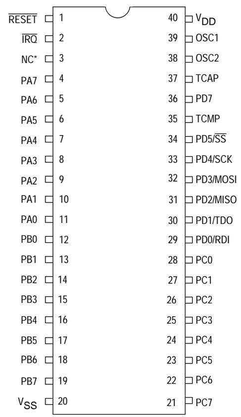
\* If MC68HC705C4A OTPs are to be used in the same application, this pin should be tied to V<sub>DD</sub>.
