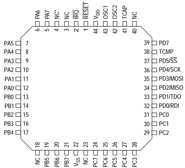
\* If MC68HC705C4A OTPs are to be used in the same application, this pin should be tied to  $V_{DD}$ .
