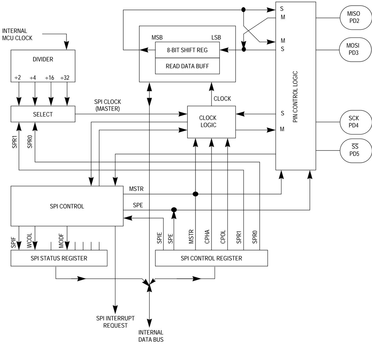
**Figure 10-2. Serial Peripheral Interface Block Diagram**
