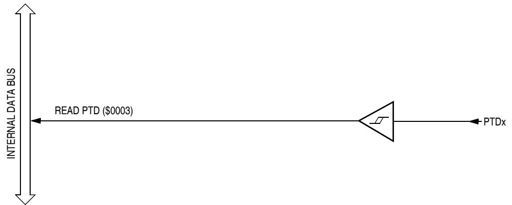
Figure 15-12. Port D Input Circuit
