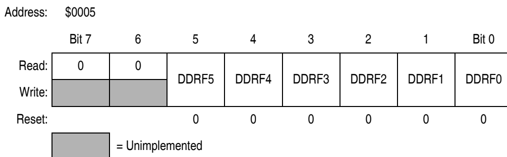
Figure 15-17. Data Direct Register F (DDRF)
