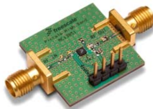
Figure 12. Typical Assembled Evaluation Board with SMA Connectors
