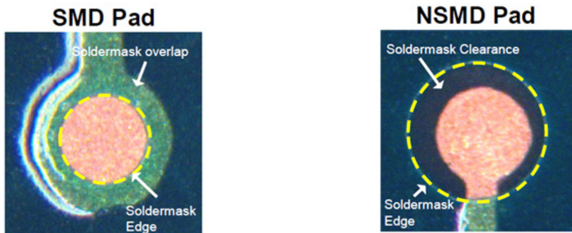
Figure 26. Solder mask (SMD) and non-solder mask defined (NSMD) pads
