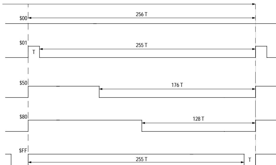
Figure 12-2 PWM output waveforms (POL = 1, active high)
