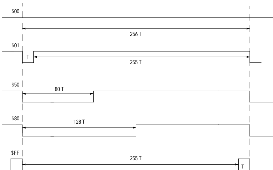
Figure 12-3 PWM waveforms (POL = 0, active low)
