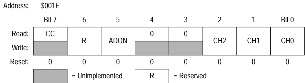
Figure 11-1. A/D Status and Control Register (ADSCR)
