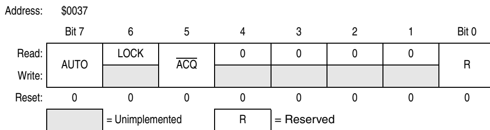
Figure 4-5. PLL Bandwidth Control Register (PBWC)
