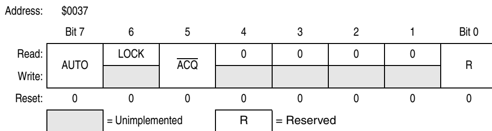
Figure 4-5. PLL Bandwidth Control Register (PBWC)
