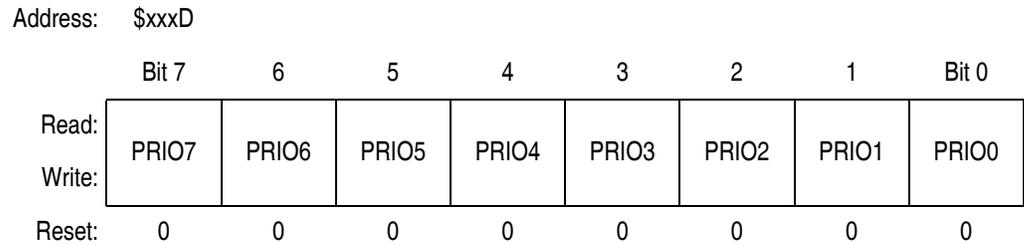
**Figure 22-12. Transmit Buffer Priority Register (TBPR)**
