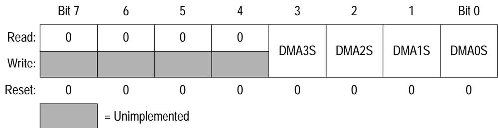
**Figure 5. TIM DMA Select Register (TDMA)**
