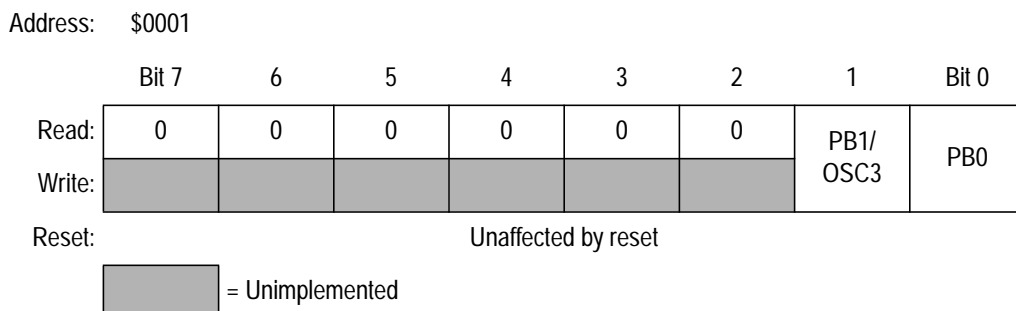
Figure 7-5. Port B Data Register (PORTB)
