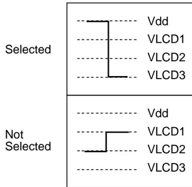
**Figure 11-5: 1/4 Duty LCD Backplane Driver Waveforms**
