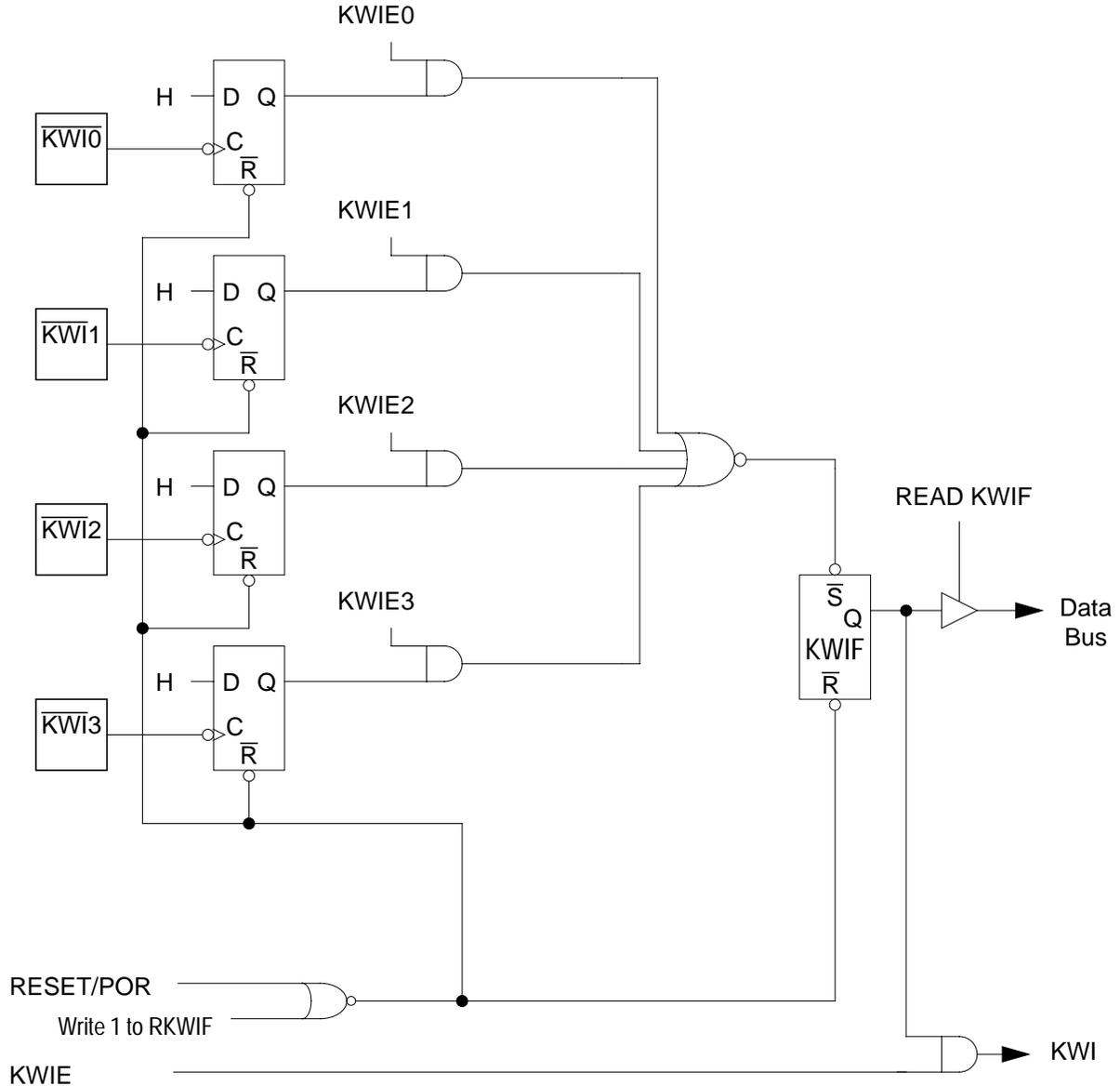
**Figure 7-10: Key Wake-up Interrupt (KWI)**
