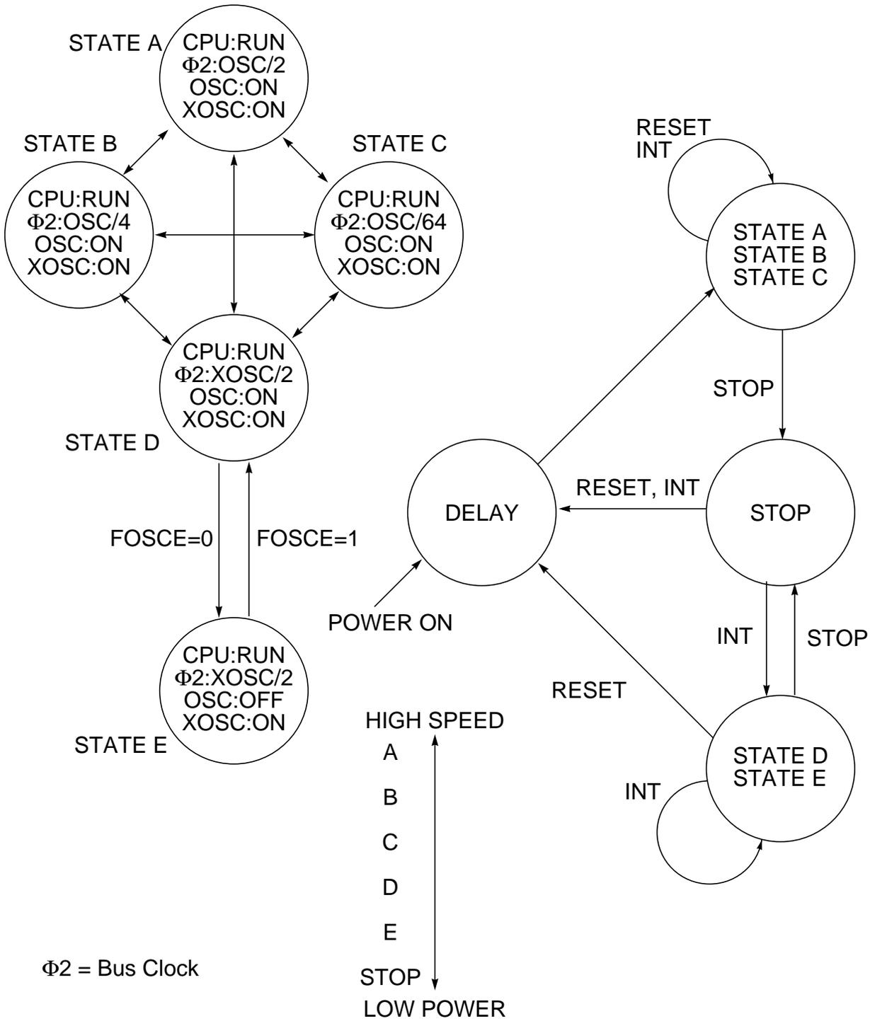
**Figure 8-4: Clock State and STOP/POD Delay Diagram**
