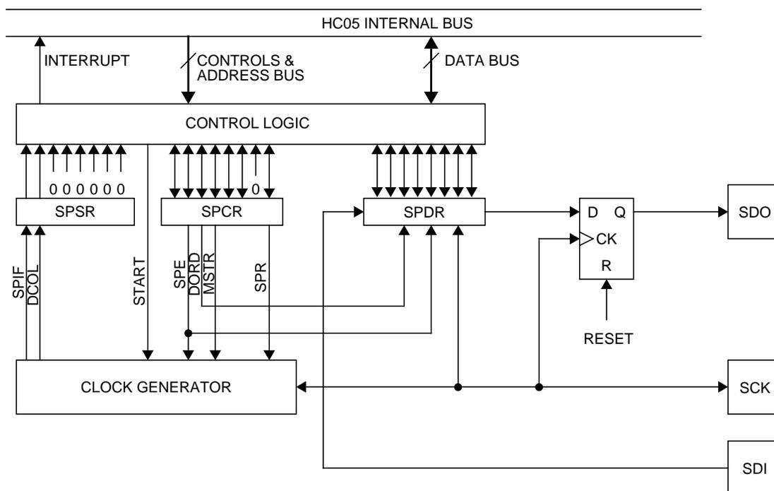
Figure 10-1: SPI Block Diagram
