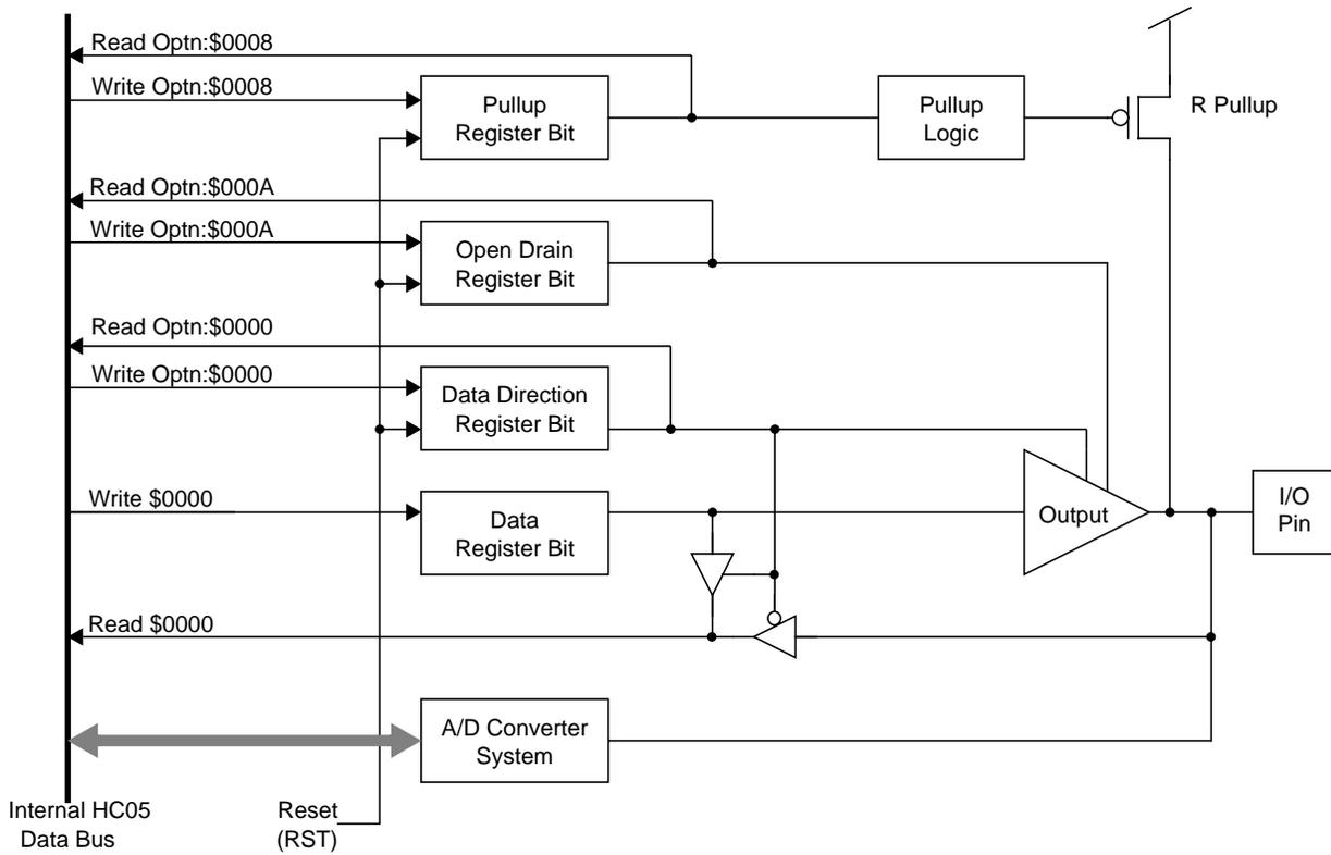
**Figure 7-5: Port A5/AD1 I/O Circuitry**
