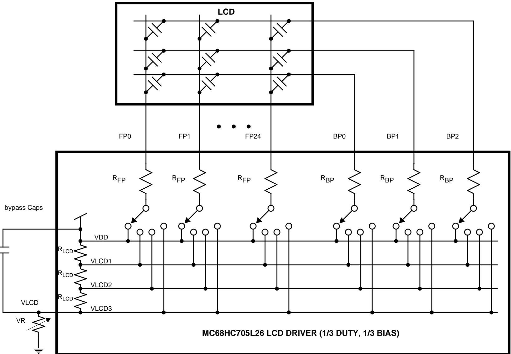
Figure 11-9: Simplified LCD Schematic
