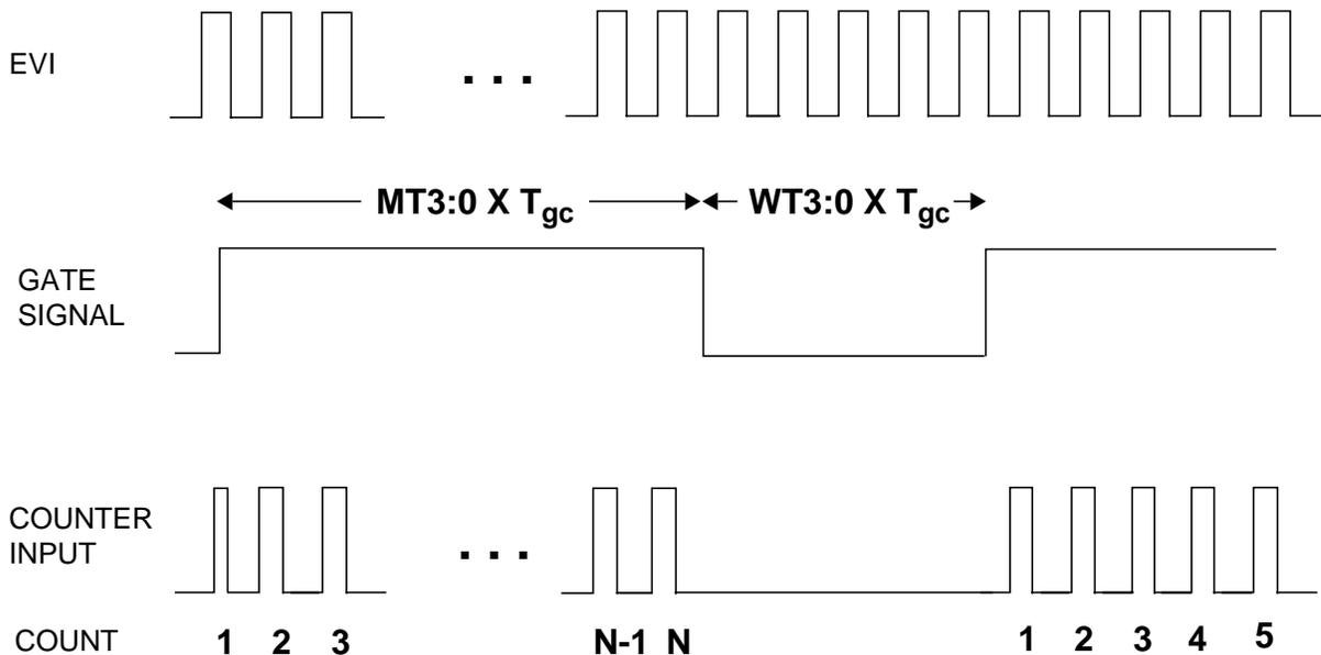
**Figure 14-4 Event Counter Input Timing Example**
