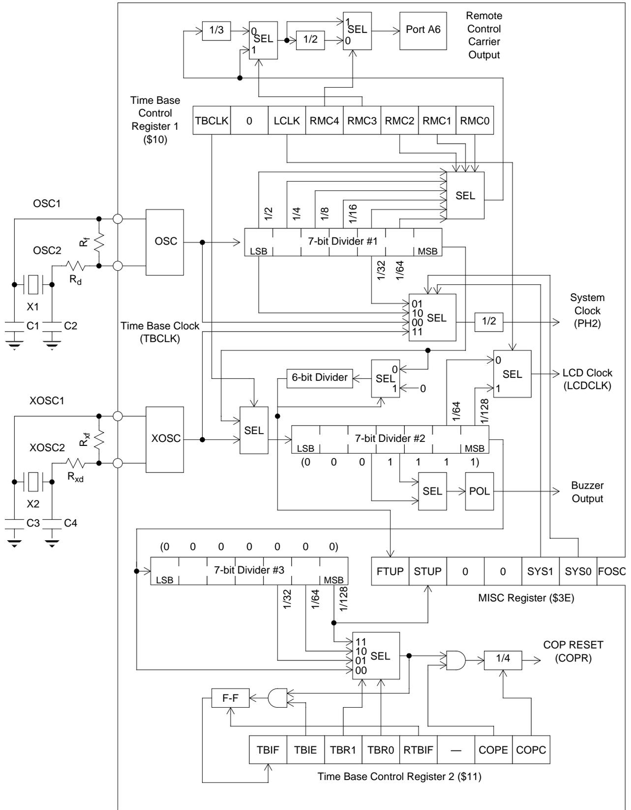
Figure 8-2: Clock Signal Distribution
