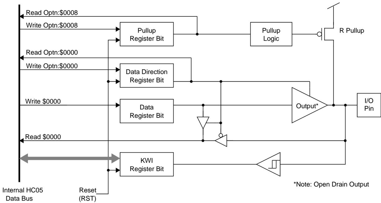
Figure 7-1: Port A0:3/KWI0:3 I/O Circuitry
