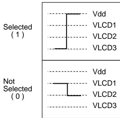
**Figure 11-7: 1/4 Duty LCD Front Plane Driver Waveforms**
