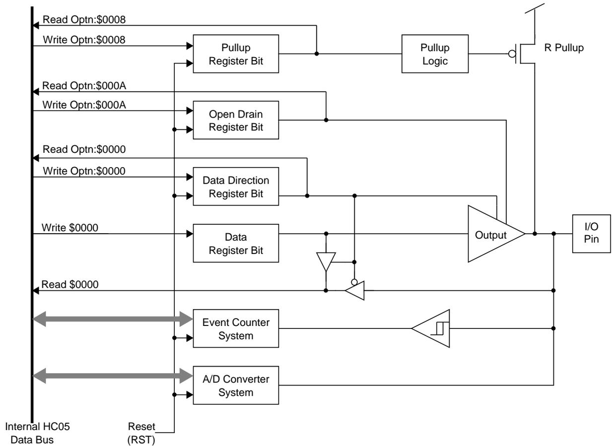
**Figure 7-4: Port A4/AD0/EVI I/O Circuitry**
