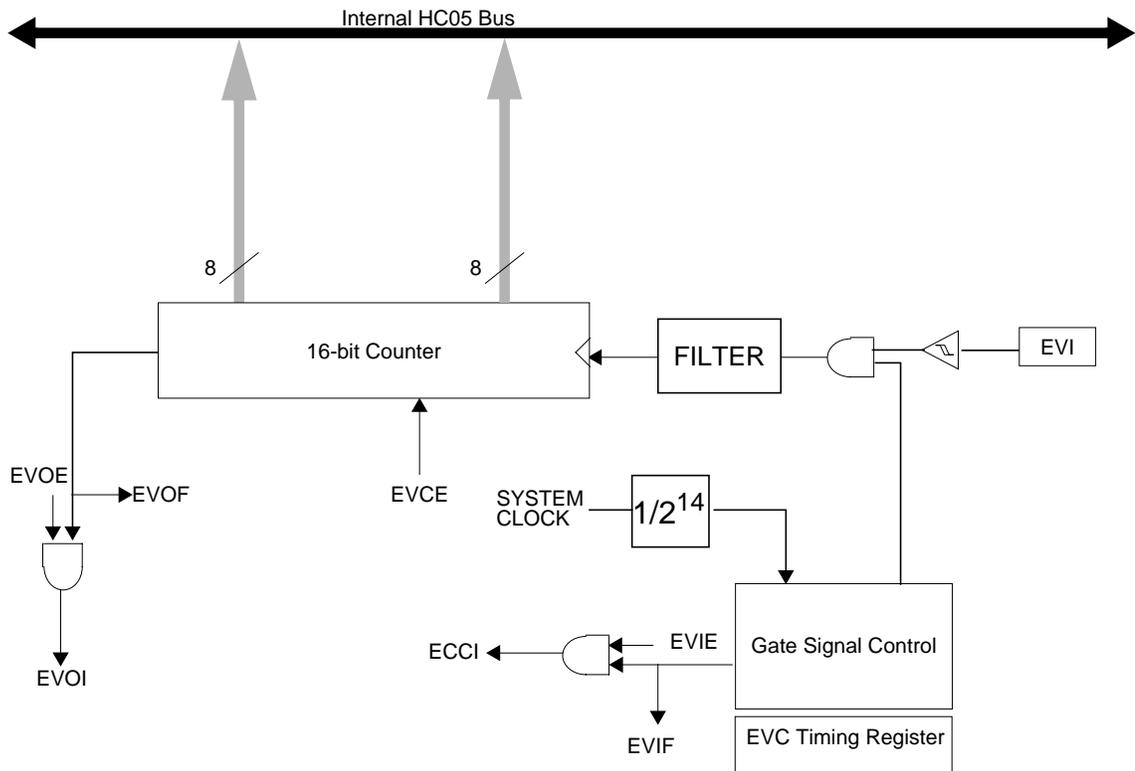
**Figure 14-1: Event Counter Block Diagram**
