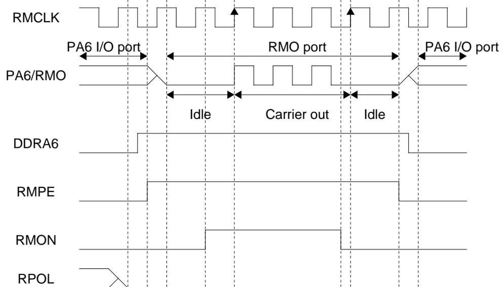
**Figure 9-2: Remote Control Carrier Output Port Control (RPOL=0)**
