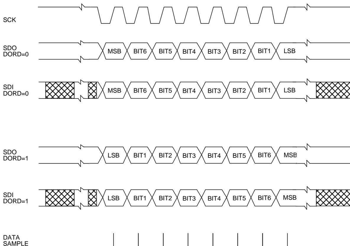
Figure 10-5: Clock/Data timing
