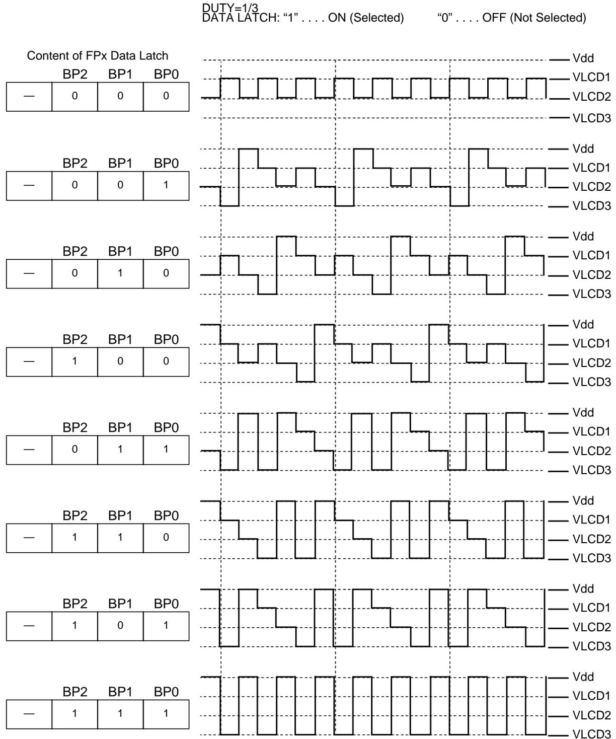
Figure 11-6: 1/3 Duty LCD Front Plane Driver Waveforms
