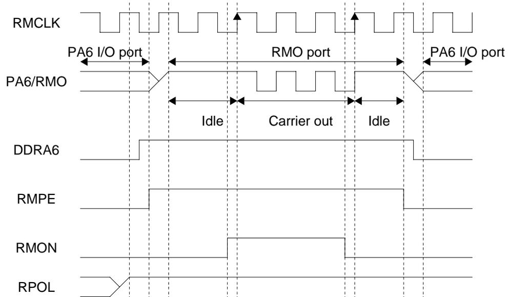
**Figure 9-1: Remote Control Carrier Output Port Control (RPOL=1)**
