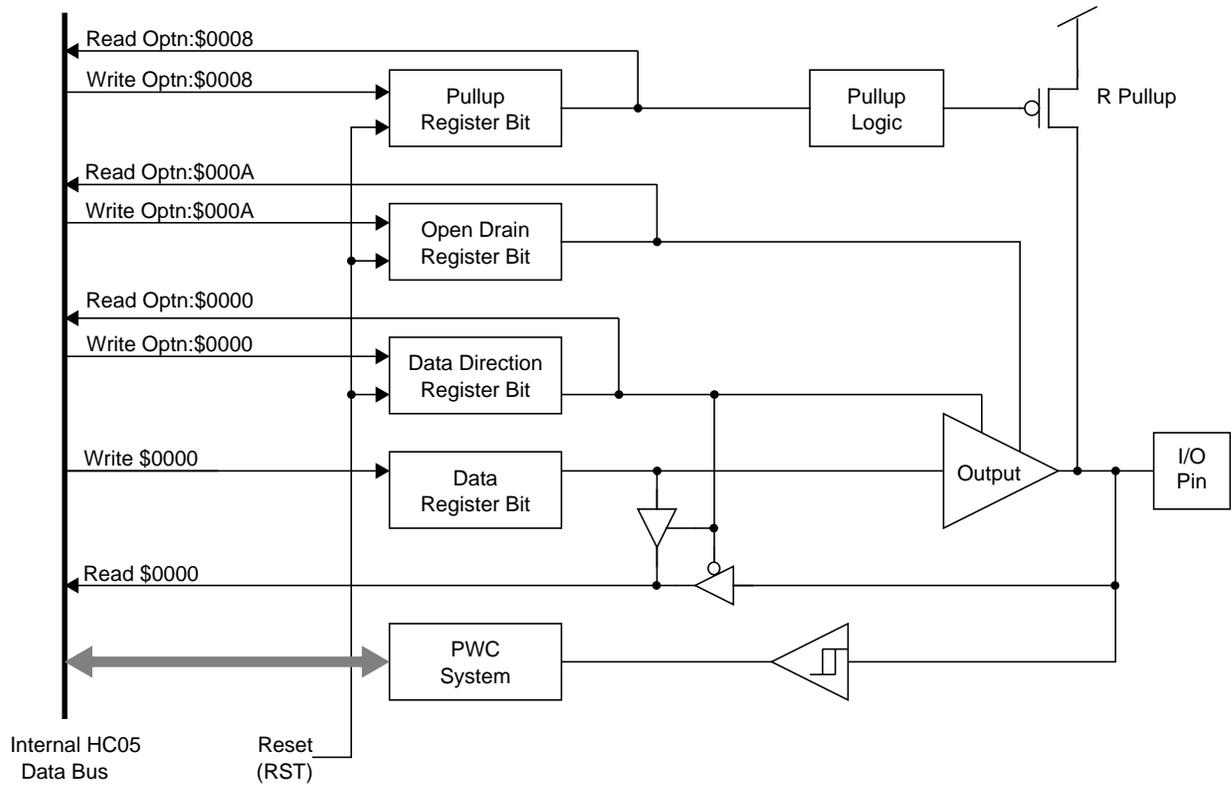
**Figure 7-7: Port A7/PWCI I/O Circuitry**
