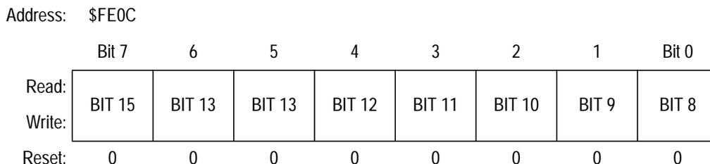
**Figure 11-4. Break Address Register (BRKH)**
