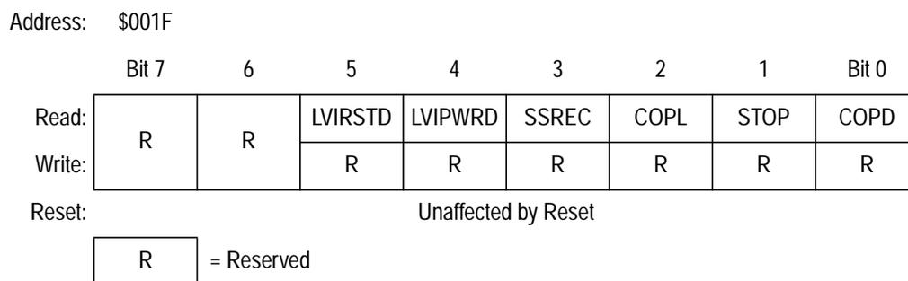
**Figure 5-1. Configuration Register (CONFIG)**
