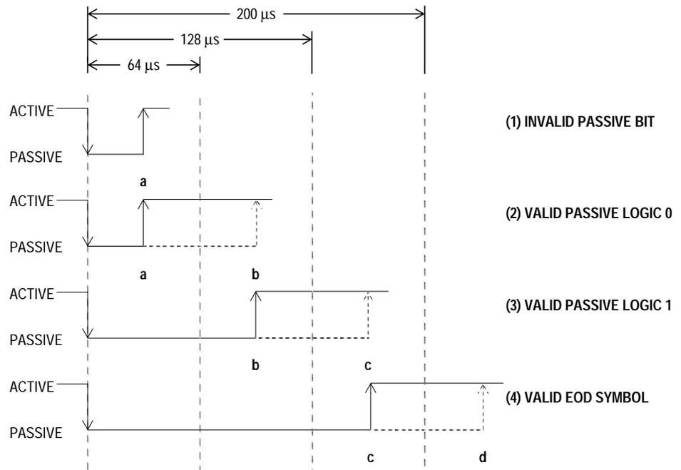
**Figure 20-8. J1850 VPW Received Passive Symbol Times**
