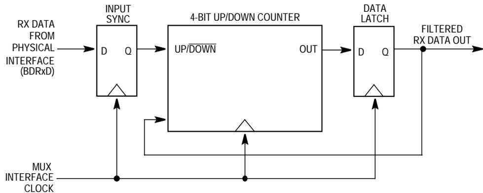
**Figure 20-5. BDLC Rx Digital Filter Block Diagram**
