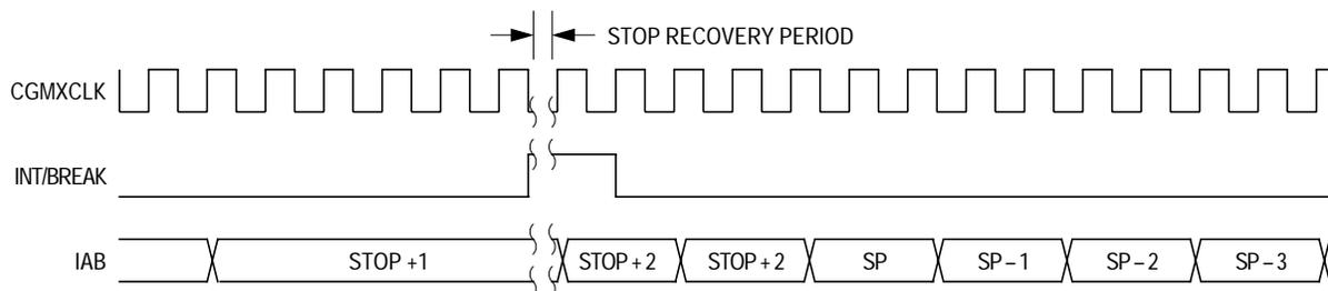
**Figure 9-16. Stop Mode Recovery from Interrupt or Break**
