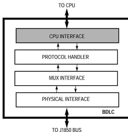
**Figure 20-15. BDLC Block Diagram**
