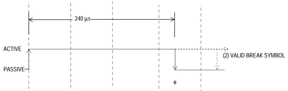
**Figure 20-11. J1850 VPW Received BREAK Symbol Times**
