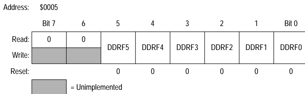
Figure 15-17. Data Direct Register F (DDRF)
