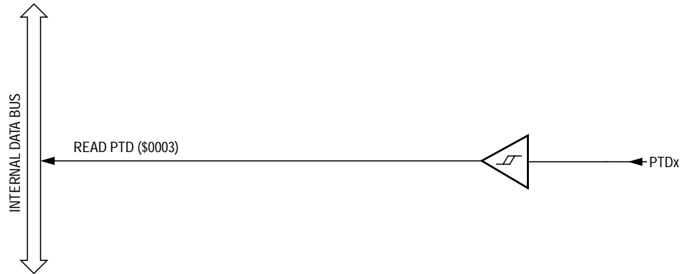
Figure 15-12. Port D Input Circuit
