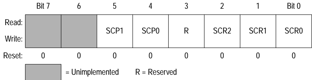
Figure 18. SCI Baud Rate Register (SCBR)
