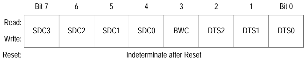
Figure 20. DMA Channel Control Registers (D0C–D2C)
