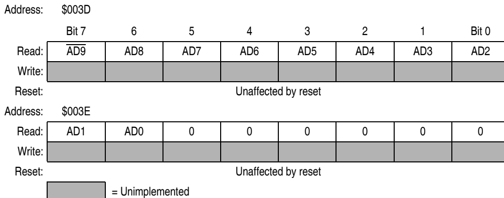
Figure 5-6. ADC Data Register High (ADRH) and Low (ADRL)
