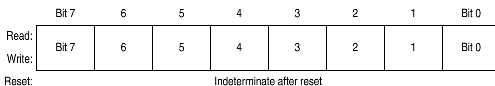
Figure 11-10. TIM Channel 0 Registers (TCH0H and TCH0L)
