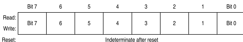
Figure 11-11. TIM Channel 1 Registers (TCH1H and TCH1L)
