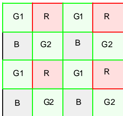
Figure 4. On-chip Bayer CFA
