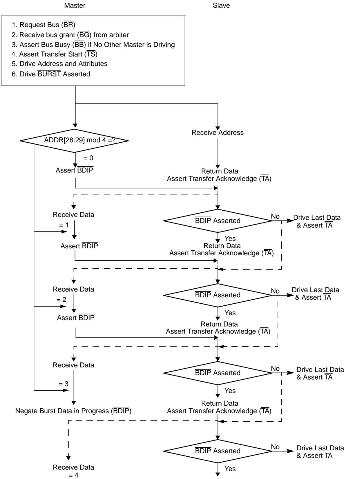
Figure 9-12. Basic Flow Diagram Of A Burst-Read Cycle
