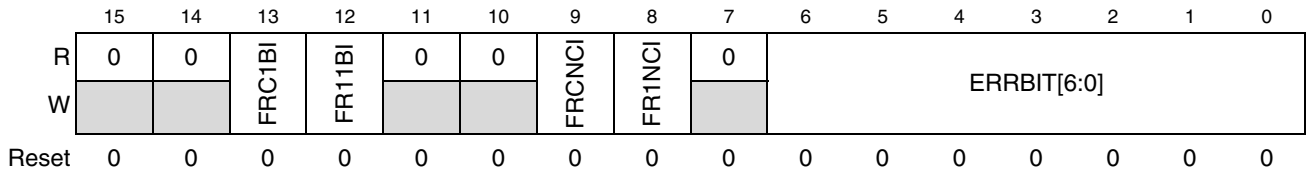
Figure 13-25. ECC Error Generation (EEGR) Register
