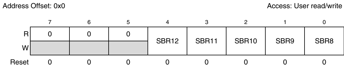
Figure 31-2. SCI Baud Rate Register High (SCIBDH)
