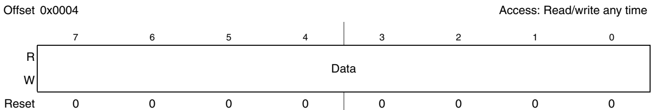
Figure 29-10. I 2 C Bus Data I/O Register (IBDR)
