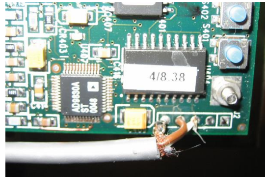
Detailed view of the RS-232 connection
