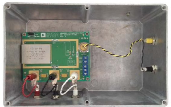
Figure 6. Metal Box (Connected to Signal Ground) Enclosing the ADA4530-1R-EBZ-BUF
