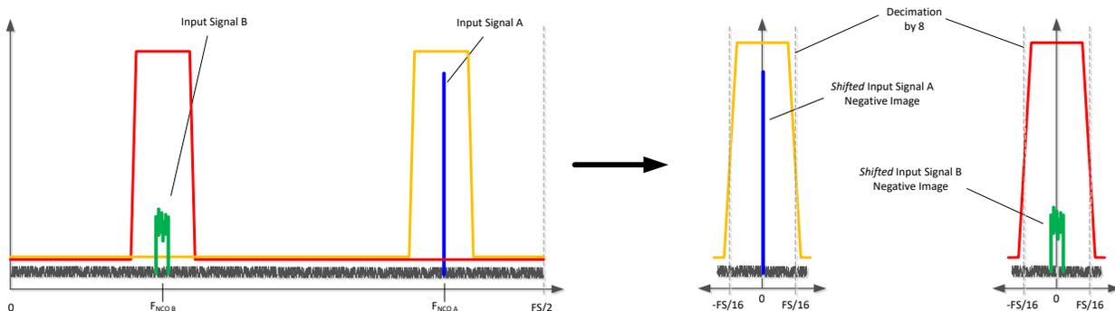
Figure 8-21. Complex Decimation (by 8) with dual band illustration
