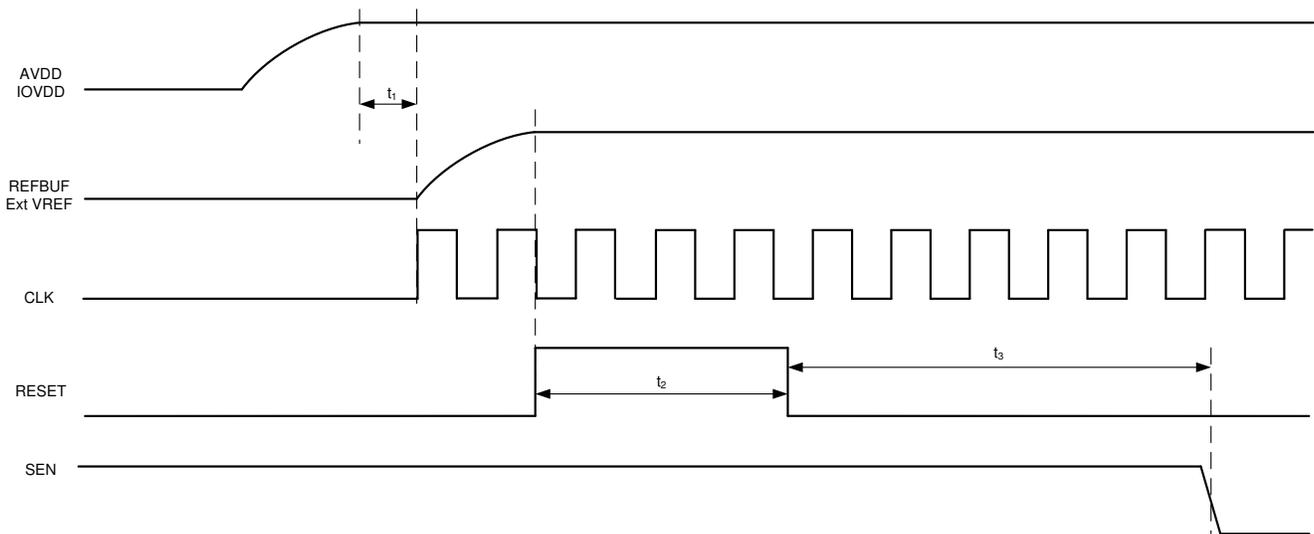
**Figure 10-1. Initialization of serial registers after power up**
