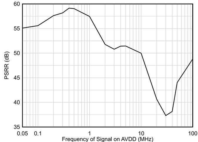
**Figure 11-1. Power supply rejection ratio (PSRR) vs frequency**
