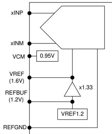
Figure 8-15. Different voltage reference options for ADC358x
