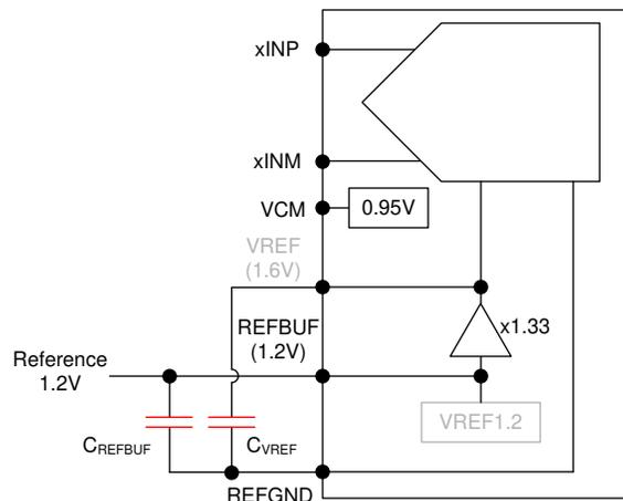
**Figure 8-18. External 1.2V reference using internal reference buffer**
