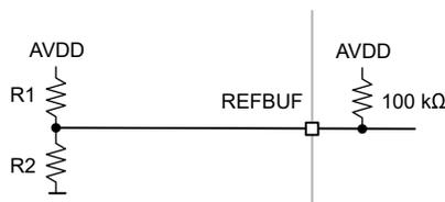
**Figure 8-41. Configuration of external voltage on REFBUF pin**
