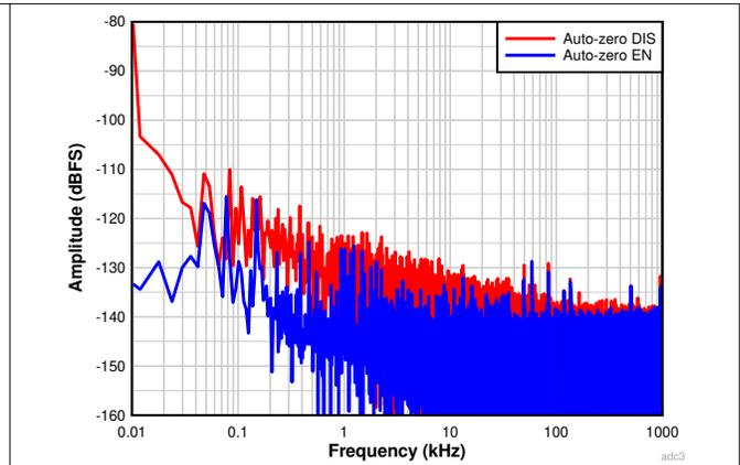
**Figure 8-9. FFT at 25 MSPS with input frequency of 3 MHz (auto-zero feature enable vs disable, 4M point FFT)**
