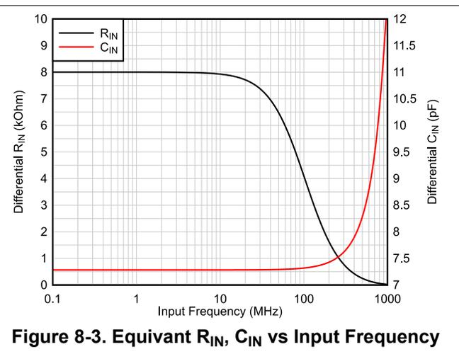
Figure 8-3. Equivalent  $R_{IN}$ ,  $C_{IN}$  vs Input Frequency
