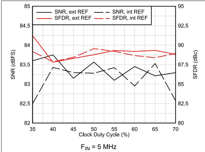
**Figure 6-19. AC Performance vs Clock Duty Cycle**
