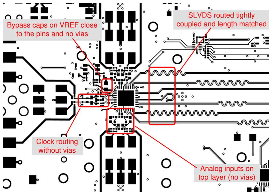
**Figure 12-1. Layout example: top layer of ADC358x/368x EVM**
