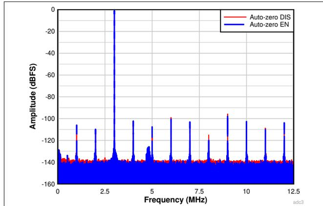
**Figure 8-8. FFT at 25 MSPS with input frequency of 3 MHz (auto-zero feature enable vs disable, 4M point FFT)**
