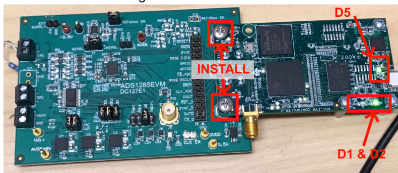
Figure 2-1. ADS1285EVM-PDK Hardware Setup and LED Indicators
