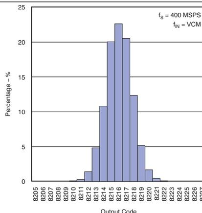
Figure 17. Noise Histogram With Inputs Shorted
