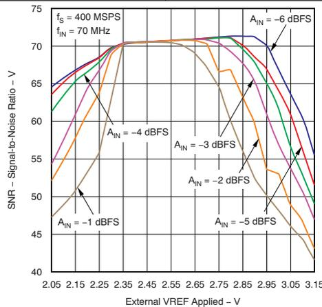
Figure 40. SNR vs External VREF and AIN
