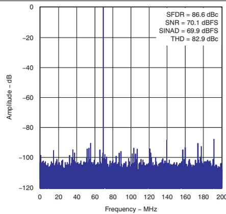
Figure 3. Spectral Performance FFT for 70 MHz Input Signal
