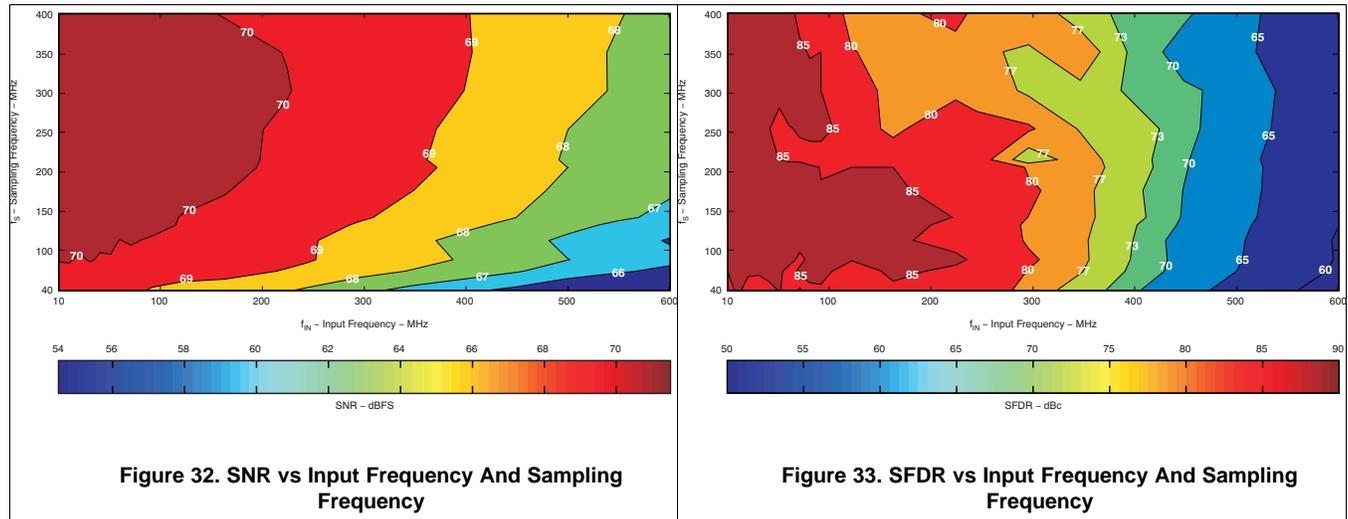
**Figure 32. SNR vs Input Frequency And Sampling Frequency**
