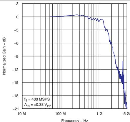
Figure 14. Normalized Gain Response vs Input Frequency
