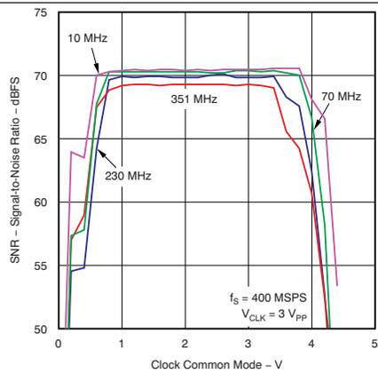
Figure 30. SNR vs Clock Common Mode
