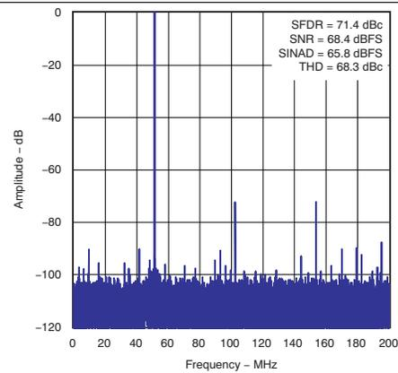
Figure 7. Spectral Performance FFT for 451 MHz Input Signal
