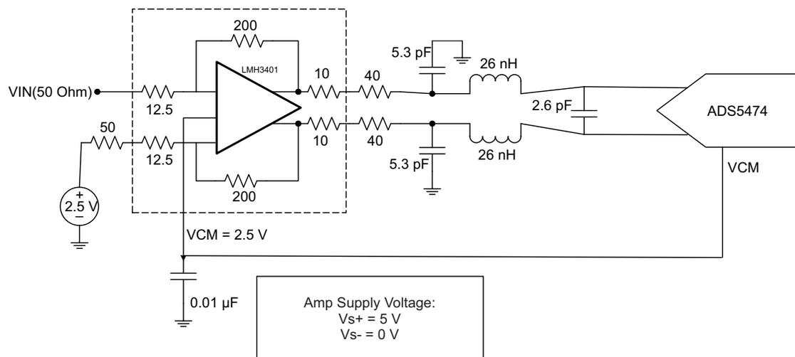
**Figure 43. Application Diagram**
