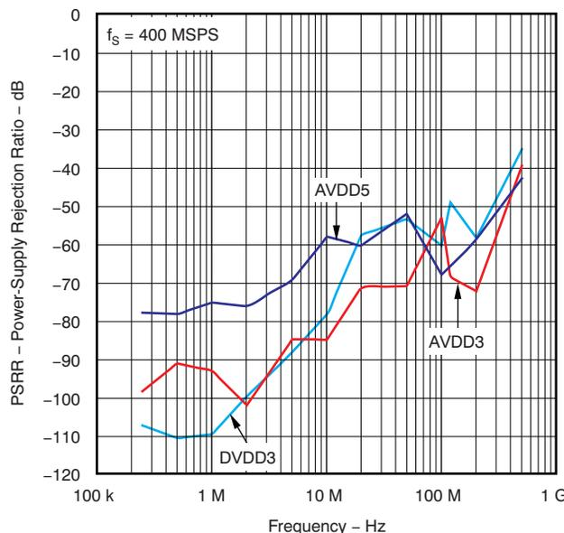
Figure 46. PSRR vs Supply Injected Frequency
