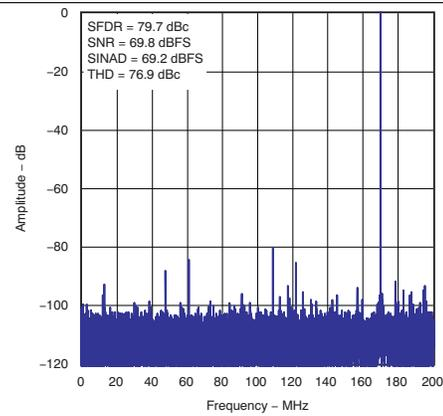
Figure 5. Spectral Performance FFT for 230 MHz Input Signal
