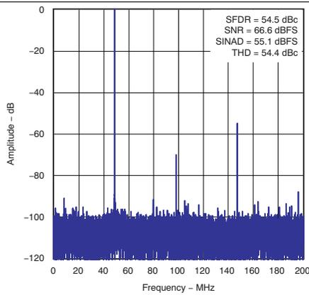
Figure 8. Spectral Performance FFT for 751 MHz Input Signal
