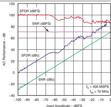
Figure 18. AC Performance vs Input Amplitude (70 MHz Input Signal)
