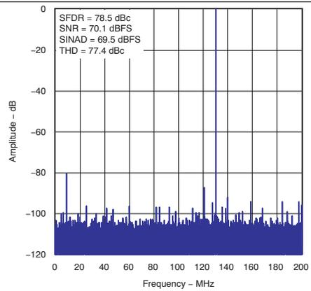
Figure 4. Spectral Performance FFT for 130 MHz Input Signal
