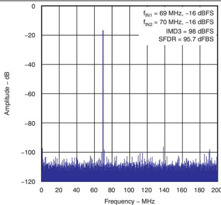
Figure 12. Two-Tone Intermodulation Distortion (FFT for 69 MHz and 70 MHz at  $-16$  dBFS)
