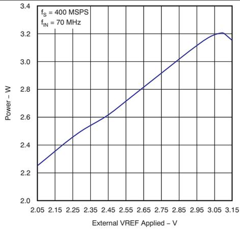
**Figure 41. Total Power Consumption vs External VREF**
