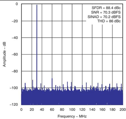
Figure 2. Spectral Performance FFT for 30 MHz Input Signal
