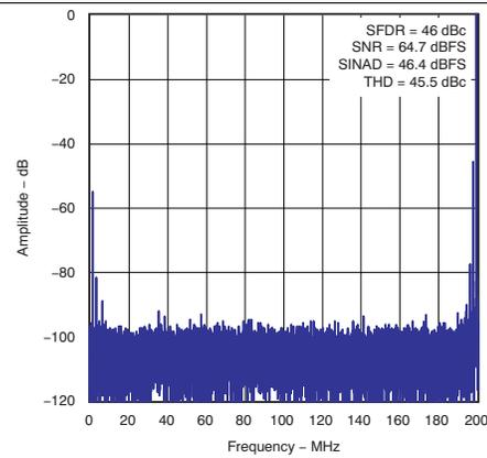
Figure 9. Spectral Performance FFT for 999 MHz Input Signal
