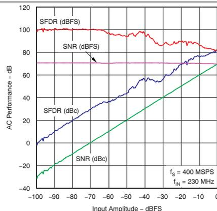
Figure 19. AC Performance vs Input Amplitude (230 MHz Input Signal)
