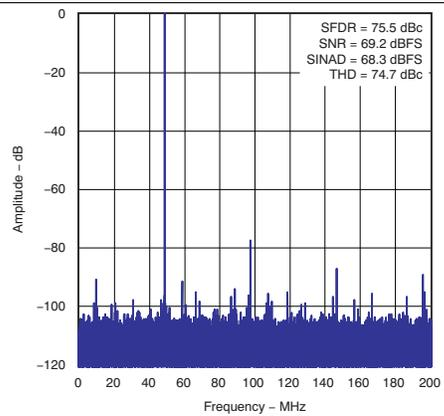
Figure 6. Spectral Performance FFT for 351 MHz Input Signal
