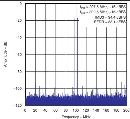
Figure 13. Two-Tone Intermodulation Distortion (FFT for 297.5 MHz and 302.5 MHz at  $-16$  dBFS)
