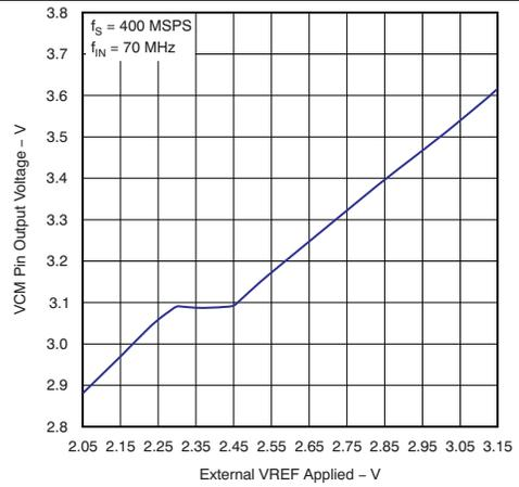
**Figure 42. VCM Pin Output vs External VREF**
