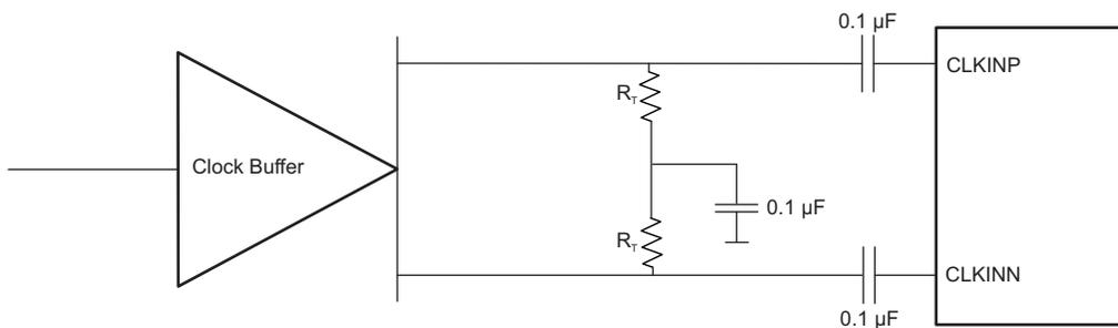
Figure 44. Recommended Differential Clock Driving Circuit
