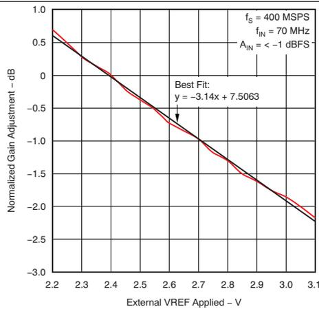
Figure 38. Signal Gain Adjustment vs External Reference (VREF)
