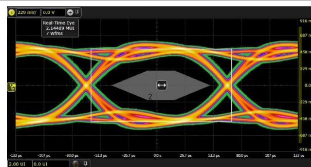
Figure 7-29. Eye at 7.5-Gbps Bit Rate with Increased Output Swing
