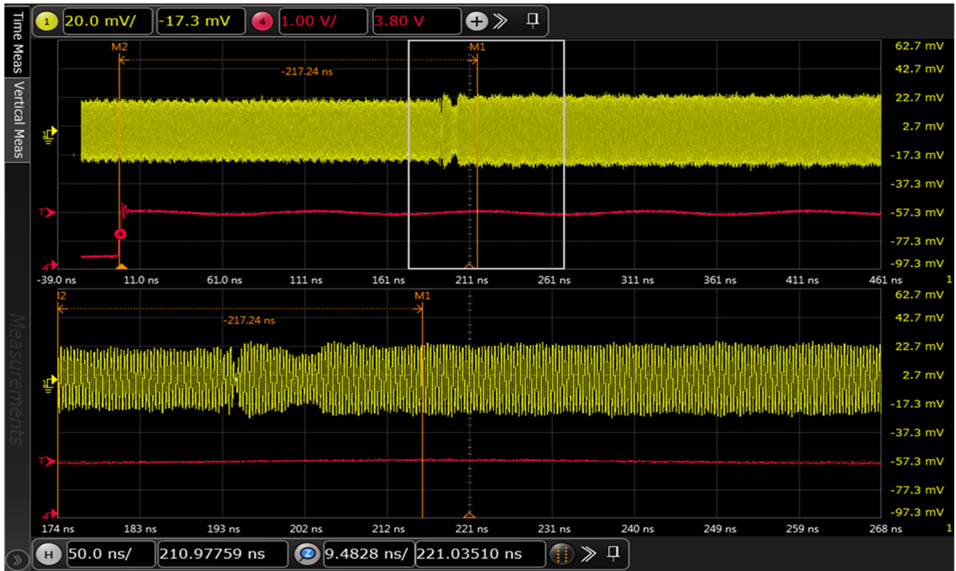
Figure 12. Scope Shot: TXA Hopping From 2200 MHz to 2800 MHz With Hop Time of 217.24 ns
