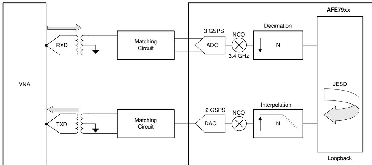
**Figure 1-1. ADC to DAC JESD Loopback**
