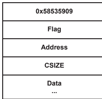
Figure 17. Compressed Section Load Command
