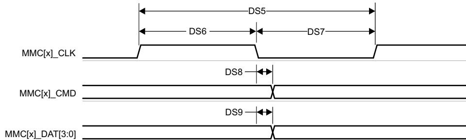
Figure 7-66. MMC1 – Default Speed – Transmit Mode
