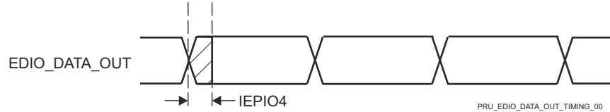
Figure 7-101. PRU_ICSSG IEP Digital IOs Timing Requirements
