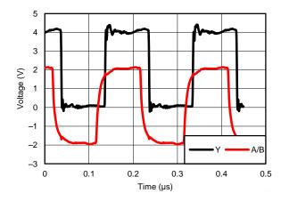
Figure 13. Differential 120- $\Omega$  Terminated Output Waveforms (Cat 5E Cable)
