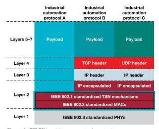
Figure 2: IEEE TSN and the communications stack.
