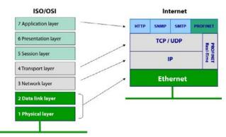
Figure 4: Industrial Ethernet protocols and Ethernet. (Source: <a href="http://profinews.com/2017/07/profinet-and-tsn/">http://profinews.com/2017/07/profinet-and-tsn/</a>).
