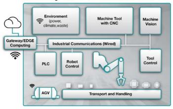
Figure 1: Industry 4.0 production cell with TSN backbone.
